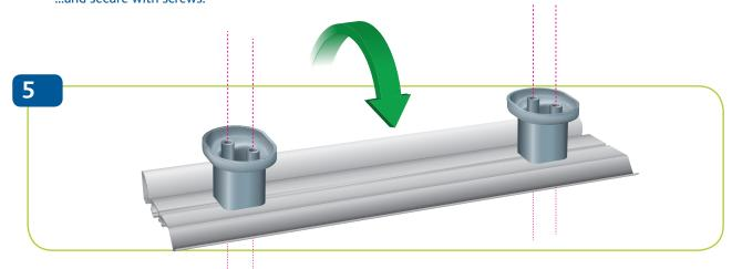
Using a 7mm drill bit, drill holes through the aluminium retainer from the back using the attached mounting brackets as guides.
